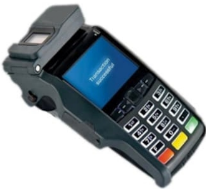
Figure 40: Micro ATM featuring a fingerprint scanner for verification...
